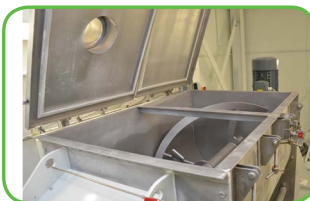
Helical Blade Mixer Interrupted spiral mixer
